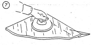
Clean pane with alcohol on both sides (Approx 2" from edge) and edge. DO NOT TOUCH SUR-FACE OF PANE WITH FINGERS AFTER CLEANING.
