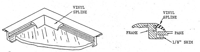
Cut vinyl spline to fit frame. Oversize 1/8" per ft. of length to allow for shrinkage of vinyl. Check miter joints for snug fit. Cut(4)- 1/8" wide sections of vinyl to be used later for Heat-Welding joints.
