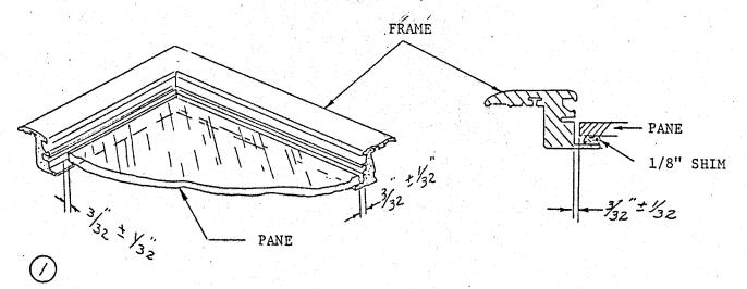
Place 1/8" soft shims along flange to prevent scratching pane. Cut window pane to fit frame. Allow 3/32" clearance between pane and frame. Flat grind and seam edges.
