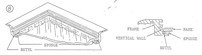
Carefully lower pane into frame making contact with Butyl. Check alignment of pane with frame for proper 1/16 - 1/8" clearance. Then apply gentle pressure along edge of pane, forcing the Butyl to "Wet" the pane and flow into and fill the space between the Neoprene Sponge and the vertical wall of the frame. The pane is to make contact with the sponge along entire surface of sponge. Damp wipe pane with alcohol, but do not puddle or allow solvent to contact Butyl. Remove guides from corners.
