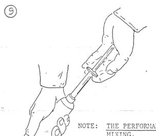
Mix 2 Part Polysulfide Sealant (PR-1221 Bl Semkit, PRC Corp.)
