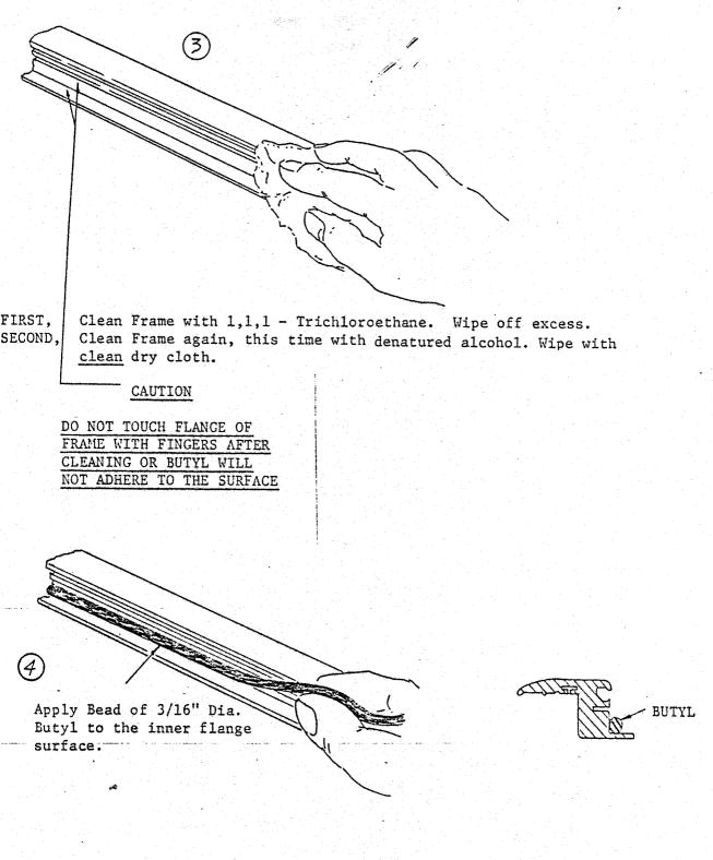
NOTE: Join successive beads using scarf joint.
